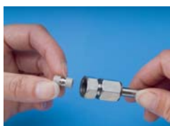
Remove the XF end fitting and install the guard cartridge in the end of the column.
