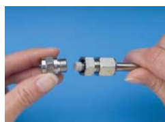
Add the XG-XF fitting (order cat.# 25026 for 10mm guard cartridges, cat.# 25062 for 20mm guard cartridges).
