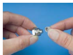
The cap frit can be easily replaced if it becomes contaminated/plugged.
