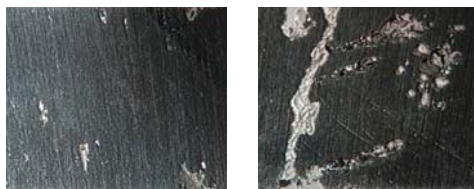
Figure 1 Silcosteel®-CR treated 316L stainless steel shows no crevice corrosion and only slight pitting corrosion, while bare 316L stainless steel exhibits severe crevice corrosion.
