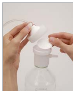
Place membrane filter on top of grid.
